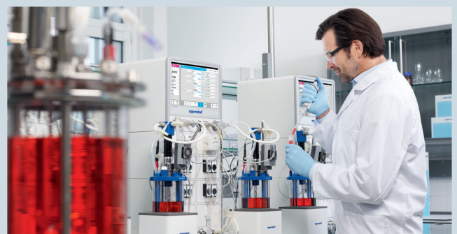
Fig. 4: AAV-2 capsids production in a batch culture using SciVario twin bioreactor control system and BioBLU 1c Single-Use Bioreactors
